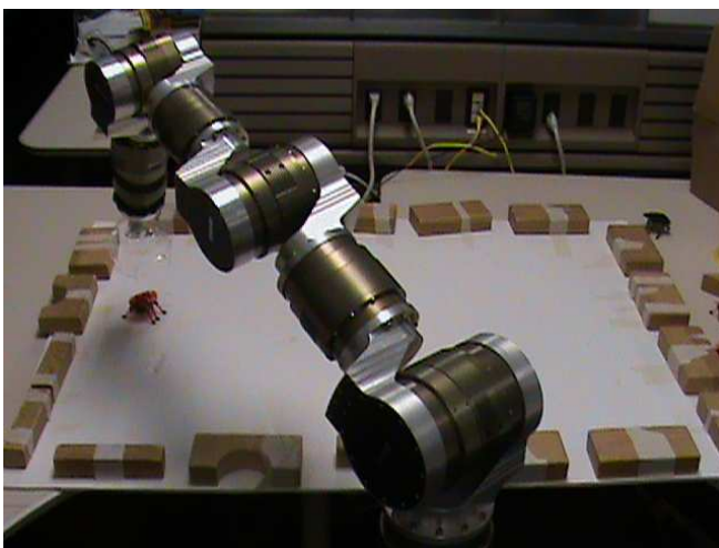
Fig. 10. Still image of robot arm converged on the x,y coordinate of a HexBug while moving in the workspace. Capture with the plastic cup pending resolution of conflict between NTCAN and Comedi
